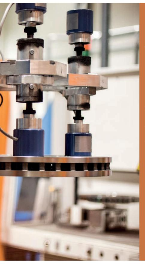
The use of **robots** in mechanical processing tasks has made it possible to automate and integrate all phases of the brake disc production process (processing, assembly, powder coating and control) into a single line.
